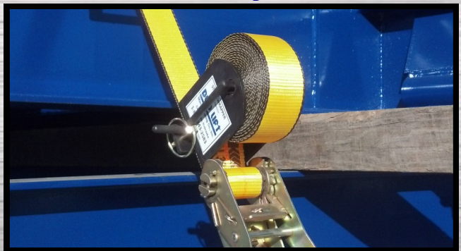
LOCK Crank Down on Strap Wrapper
