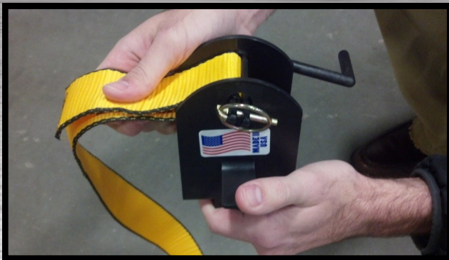
FEED Strap into Crank
